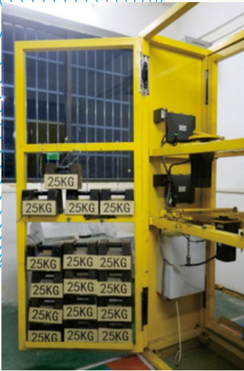
790 lbs (360 kg) Load-Bearing Test
