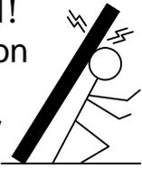
TIGHTEN set-screws to eliminate mullion channel rattle or looseness
