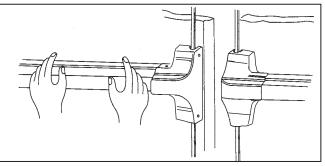
3. Turn and adjust upper connecting tube until top latch assembly retracts properly and then fix the connecting pin by bending 2 ends.
