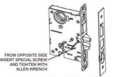
Reinstall the special screw and tighten securely with the provided allen wrench.
