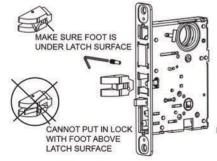
3. Rotate Latch bolt 180° and reinstall into lock, pushing the latch bolt into the lock and then releasing.
