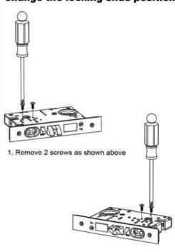
Turn lock over to oppcsite side and reinstall screws as shown above.
