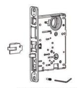
2. Pull latch bolt out of lock
