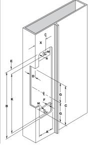
**RCI 7105, 7305** Aluminum & Wood Frames, 1-1/2" D **RCI 4105, 4305** Aluminum & Wood Frames, 1-1/2" D Any modular **A41, A43, A71** or **A73** with **B4705** faceplate
