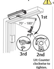
Keep door open in position until dial screw secures dial.
