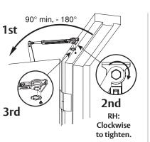
Keep door open in position until dial screw secures dial.
