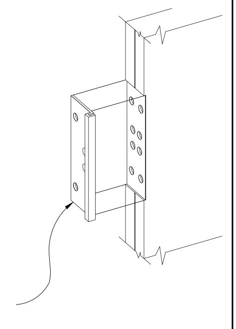
.027" (0.7mm) ADAPTER USED WITH .180" (4.6mm) 4-1/2" (114.3mm) OR 5" (127.0mm) HINGE
