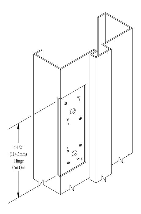
4 Projection dimples marked ( X ) are added to hinge reinforcement for standard 4-1/2" x 4-1/2" full mortised template hinge .134 thickness.
