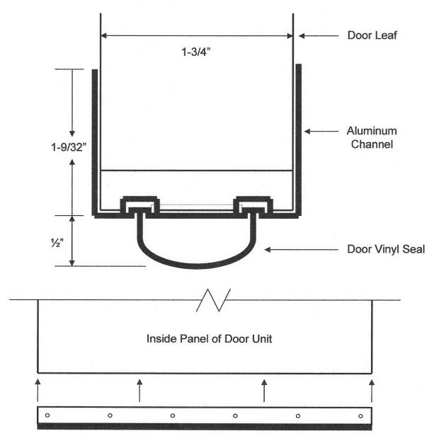
Door Bottom Seal Aluminum Channel is Installed with Screws to the Inside Skin of the Door Leaf to Prevent Corrosion
