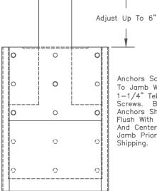
Anchors Screwed To Jamb With #10 1-1/4" Tek Screws. Both Anchors Should Be Flush With Ends And Centered In Jamb Prior To Shipping.
