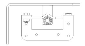
NOTE: BRACKET MOUNTS ON TOP OF BEARING PLATE
