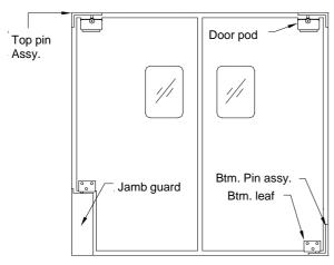
NOTE: Bottom pin assembly must be secured to floor
