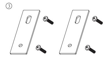
SHIM (2PCS) AND 1/4"x1" ROUND HEAD SCREWS (4PCS) FOR TOP AND BOTTOM LATCH UNIT.
