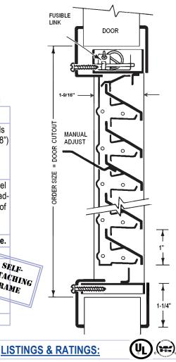
Fire Ratings with UL & WHI Classification Marks Tested & Listed for UL10C, and classified in accordance with UBC7-2-94, ASTM E152, CAN/ULC S104, NFPA 252. Install in accordance with NFPA80.
