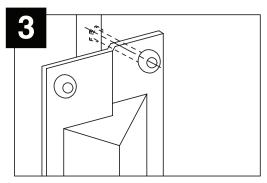
Fasten to door using two supplied carriage bolts and hex nuts.
