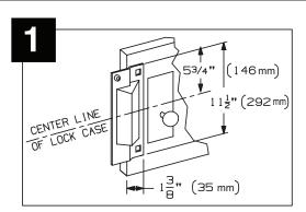
Locate lock guard as shown, making sure to center with the lock case.
