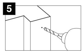
Drill 5/16" (8mm) hole in the frame to accept security pin.
