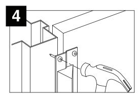
Swing door closed until security pin touches the frame. Mark hole location by hitting head of security pin with hammer.
