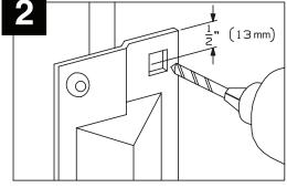
While holding lock guard firmly against door, drill two 5/16" (8mm) diameter mounting holes.
